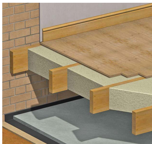
Figure 03: insulating / refurbishing ground floors
