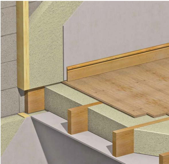
Figure 04: insulating / refurbishing walls and intermediate floors
