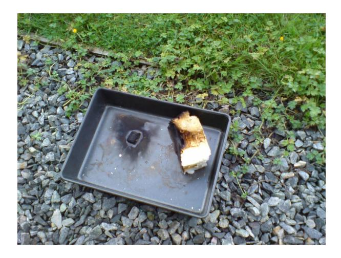
These results show that although Icynene is classed as a combustible material by the BBA, in the simple tests carried out for this report it performed very well as a fire break, resisting the spread of fire and slowing the heat transfer rate significantly. These trends should be replicated when the BS EN 13823:2002 (single burning item) or BS EN 11925-2 (small flame ignitability) have been carried out and fully validated results are produced.
