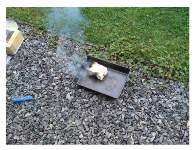
It was found during this test that the Icynene had a smothering effect on the fire, and although initially the outer face of the sample became quite heavily charred, the fire did not penetrate the sample.
