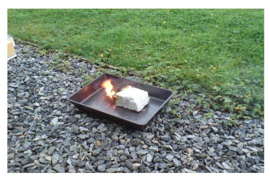
After a short space of time in close proximity to the fire the test sample of Icynene developed a hard black layer that proved to be fairly impenetrable by fire, after a further 5 minutes the fire had spread no further in to the test sample.
